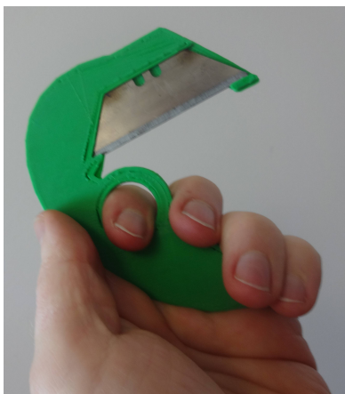
Figure 12. A dressing tool that mounts a replaceable utility blade on a 3-D printed handle with a guard.
