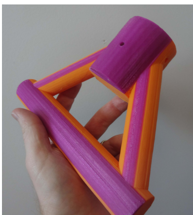
Figure 3. A 3-D printable customizable shovel handle in which the color of the filament had been switched during the print for cosmetic reasons.
