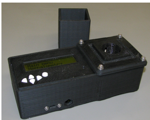
Figure 6. 3-D printable open-source mobile water quality testing platform capable of both colorimetry for biochemical oxygen demand/chemical oxygen demand and nephelometry.
