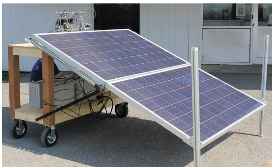
Figure 1. a) Community-scale PV-powered open-source RepRap 3-D printer system for off-grid community use and b) the basic schematic design. The PV are connected in parallel; a combiner box is used to combine and drive the DC supply towards a 30 A charge controller, which maintains the controlled charging and discharging of the batteries. The batteries are connected in two parallel lines with each line containing two unit cells in series. During charging periods four 120 AH batteries are fed DC current while discharging continues to power the RepRap and the laptop through a DC/AC inverter.
